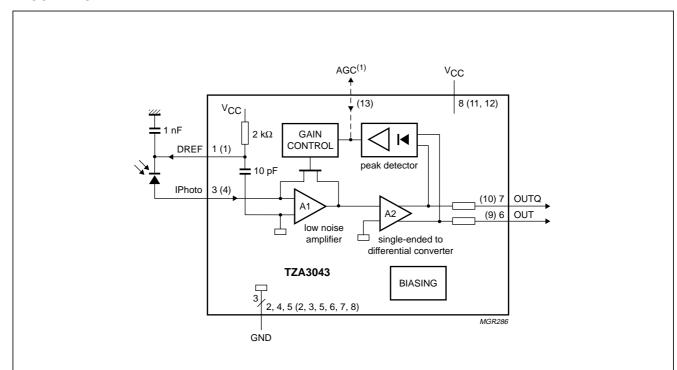
(1) AGC analog I/O is only available on the TZA3043U (pad 13). The numbers in brackets refer to the pad numbers of the naked die version.
